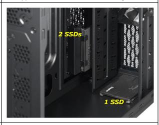
Supports up to 3 SSDs - 2 on the tool-less cage, 1 at the bottom of HDD cage
